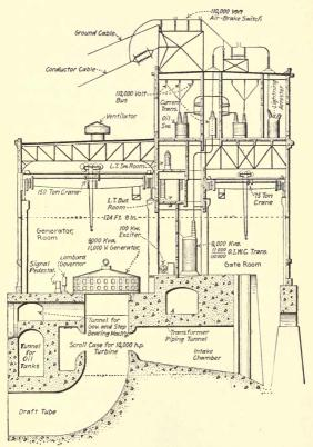
Fig. 300.—Sectional elevation of the Keokuk hydro-electric station.
